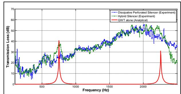
Figure 13: Transmission Loss comparison of dissipative perforated tube, hybrid silencer and QWT (QWT length = 100 mm)
