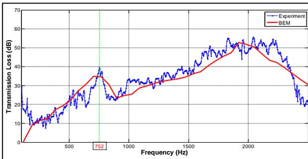
Figure 11: Transmission Loss of Hybrid Silencer with 100 mm length of QWT ( $d_h = 4$  mm and  $\phi = 28.8\%$ )
