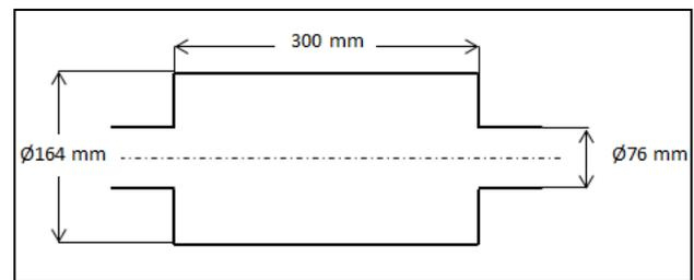
Figure 4: The schematic view of simple expansion chamber
