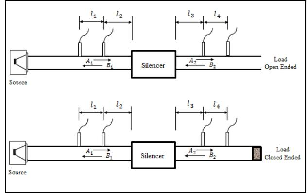
Figure 2: Schematic view of measurement setup of two load method
