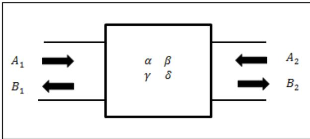
Figure 1: Transfer matrix between incident and reflecting waves
