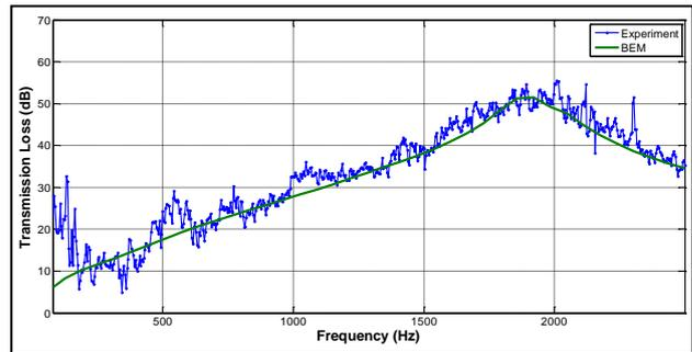
Figure 9: Transmission Loss of dissipative perforated silencer ( $d_h = 4$  mm and  $\phi = 28.8\%$ )
