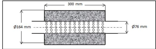
Figure 8: The schematic view of dissipative perforated silencer.
