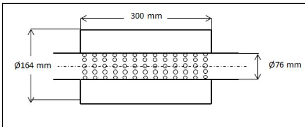
Figure 6: The schematic view of reactive perforated silencer.
