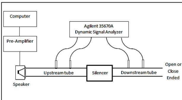
Figure 3: Schematic view of experimental test setup
