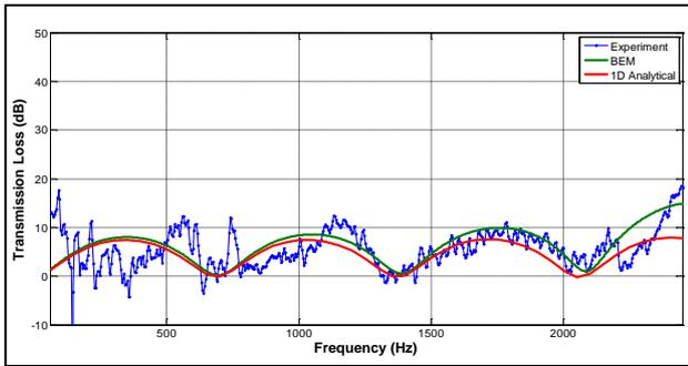
Figure 5: Transmission Loss of simple expansion chamber
