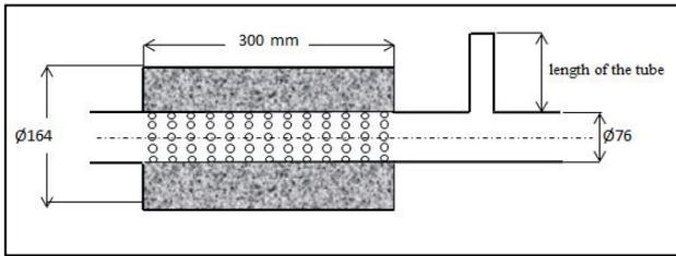
Figure 10: The schematic view of hybrid silencer
