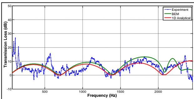
Figure 7: Transmission Loss of reactive perforated tube with  $d_h = 4$  mm and  $\phi = 28.8\%$  (Staggered array)
