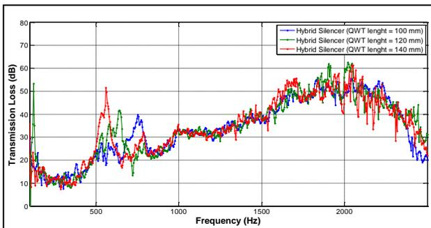
Figure 12: Transmission Loss of Hybrid Silencers (Experiment)
