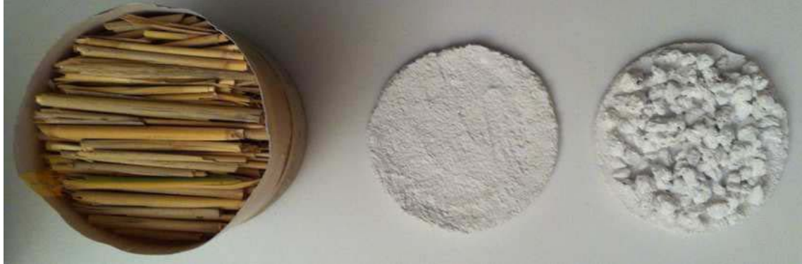
FIGURE 4. The Layer of Configurations: Reed, Pumice Powder&Lime, Pumice Stone& Lime
