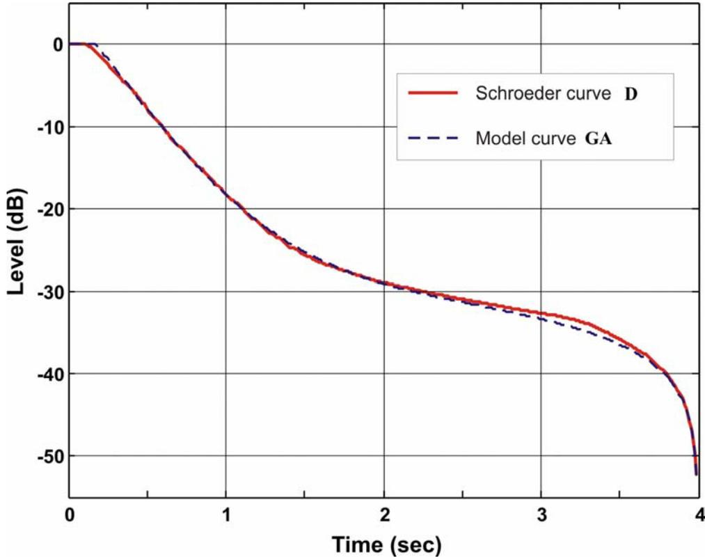
*Figure 1. Schroeder decay function measured in Sant. Patrick Church, Watervliet, NY, along with the decay model function.*
