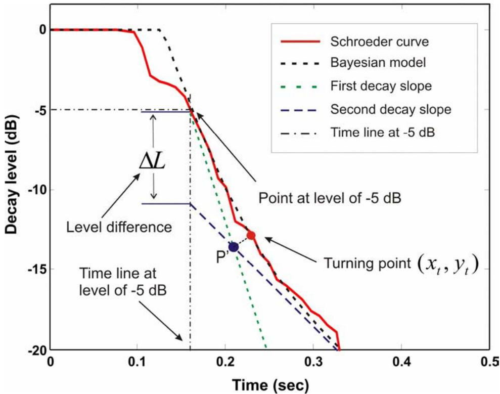
**Figure 3.** Definition of level difference  $\Delta L$  and turning point  $(x_t, y_t)$  with help of a zoom into a small portion of Fig. 2.
