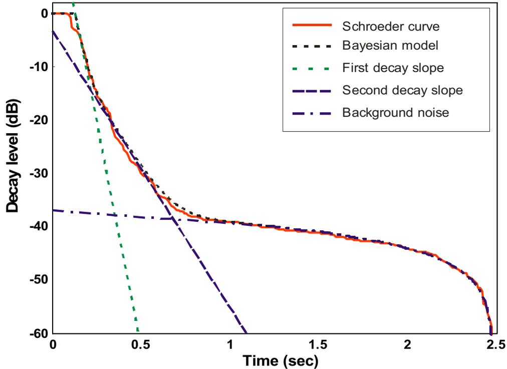
**Figure 2.** Comparison between measured decay function (Schroeder curve) in scale model coupled spaces and the decay model function. The model function is decomposed into 3 terms: 1<sup>st</sup> slope, 2<sup>nd</sup> slope and the term associated with background noise.
